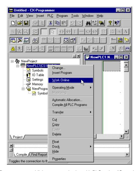
When CX-Programmer establishes communication with PLC, select "Operating Mode" (from PLC's menu) and set "Program" mode.
